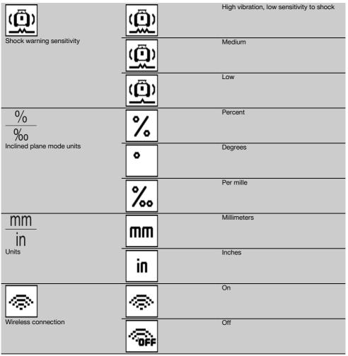
Settings that affect the rotating laser only become effective when the rotating laser is switched on and a wireless connection has been established. Pressing the "Back" key takes you back to the main menu.
